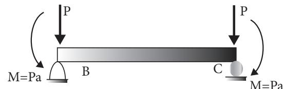
Segment BC subjected to pure bending as no shear force exists between B to C.
