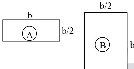
By using flexural formula,  $\sigma = \frac{M}{Z}$
