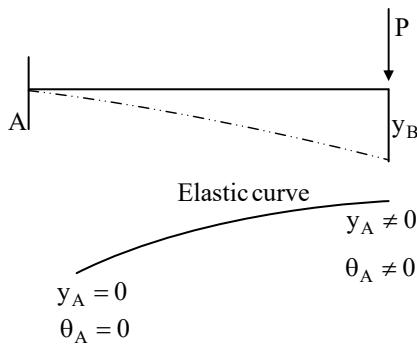
From the above diagram bending moment or stress is maximum at fixed end.
