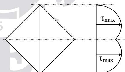
From the above diagram, the shear force distribution across the section of beam will be zero at top and bottom.
