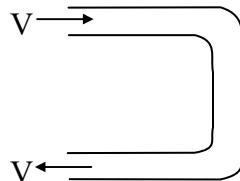
$$F_x = \rho a V (V_{1x} - V_{2x})$$
