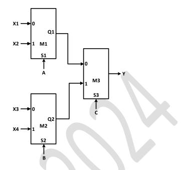
For an instance of inputs X1=1, X2=1, X3=0, and X4=0, the number of combinations of A, B, C that give the output Y=1 is \_\_\_\_\_
