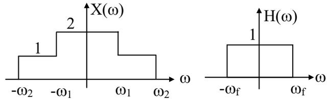
(a)  $0 < \omega_f < \omega_1 \quad Y(\omega) = X(\omega) \cdot H(\omega)$
