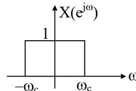
$E = \frac{1}{2\pi} \int_{-\omega_c}^{\omega_c} 1 d\omega = \frac{\omega_c}{\pi}$
