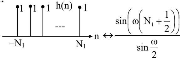
$$(a) H(\omega) = \frac{\sin\left(\frac{7\omega}{2}\right)}{\sin\left(\frac{\omega}{2}\right)}$$
