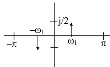
$$X(e^{j\omega}) = \frac{-j}{2}\delta(\omega + \omega_1) + \frac{j}{2}\delta(\omega - \omega_1)$$
