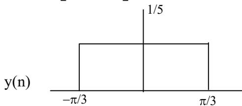
$$\sum_{n=-\infty}^{\infty} \frac{\sin \frac{n\pi}{4}}{2\pi n} \times \frac{\sin \frac{n\pi}{3}}{5\pi n} = \frac{1}{2\pi} \int_{-\pi/4}^{\pi/4} \left(\frac{1}{2}\right) \left(\frac{1}{5}\right) d\omega$$
