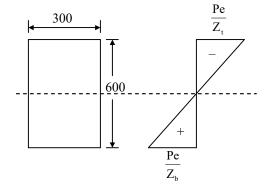
$$\sigma_b = \frac{P}{A} + \frac{Pe}{z} - \dots (1)$$
