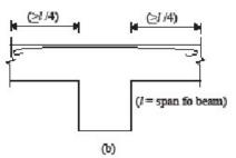
Detailing of flanged beams to ensure integral action of slab and beam
