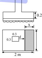
One way shear  $V_u = q_0$  [hatched area]  $= 80[0.65 \times 2] = 104 \text{ kN}$
