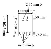
$$b = 300 \text{ mm}, D = 500 \text{ mm}, d = 462.5 \text{ mm}$$
