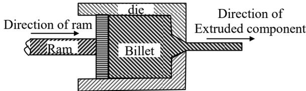
Fig. Forward extrusion
