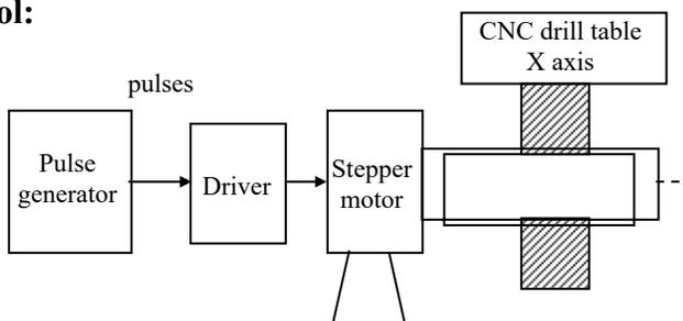
BLU = the distance traveled by the table for one pulse of electrical energy input to the motor.
