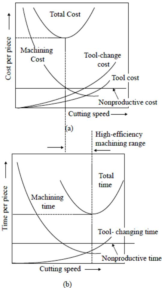
As shown in above figure, as the cutting speed increases, the cost of production initially reduces, then after an optimum cutting speed it increases. For higher feed rate the cost of production reduces for same cutting speed, but the surface finish will suffer.
