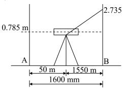
C.S.R on B =  $2.735 - 0.06735 \times 1.55^{2}$ = 2.573 m T.R.L difference between A & B = 2.573 - 0.785
