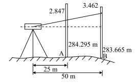
Difference in staff reading = 3.462 - 2.847= 0.615 m Difference in R.L. = 284.295 - 283.665 m = 0.63 m Difference of the above = 0.615 - 0.63= 0.015 m
