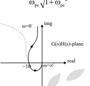
The mapping of the section  $C_1$  is shown figure.
