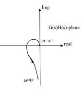
Mapping of section C<sub>4</sub>: It is the radius 'ε' semicircle, therefore sub  $s = \text{Lim} \, \epsilon e^{j\theta}$
