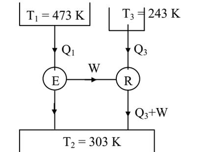
$$\eta_E = \frac{T_1 - T_2}{T_1} = \frac{W}{Q_1}$$
