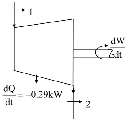
Applying steady flow energy equations
