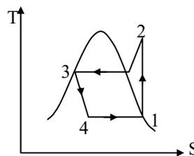
Ideal vapour compression means the compression starts from dry and saturated vapor line.
