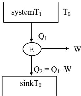
For maximum work done condition the engine has to be reversible and for the condition of reversibility entropy change of universe is zero.
