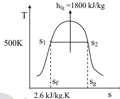
$$s_g - s_f = \frac{h_{fg}}{T_{\text{sat}}}$$
