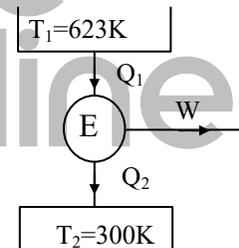
$$\eta_{\text{Carnot}} = \frac{T_1 - T_2}{T_1} = \frac{623 - 300}{623} = 0.518$$
