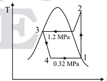
$$h_3 = 117.71 \text{ kJ/kg at } 1.2 \text{ MPa}$$
