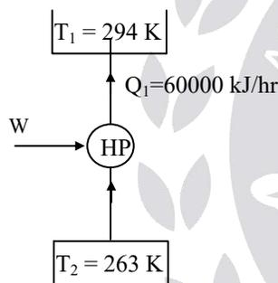
$$(\text{COP})_{\text{H.P.}} = \frac{Q_1}{W} = \frac{T_1}{T_1 - T_2}$$
