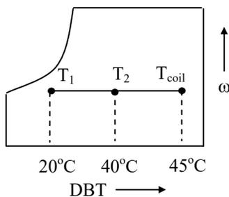
$$\text{By pass factor} = \frac{T_{\text{coil}} - T_2}{T_{\text{coil}} - T_1} = \frac{45 - 40}{45 - 20}$$
