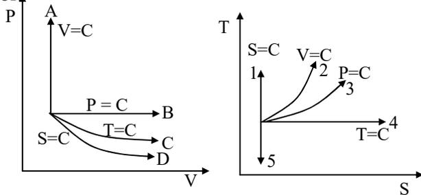
Slope of constant volume curve is more than that of constant pressure curve in T-S diagram. Similarly slope of adiabatic curve is more than that of isothermal curve in P-V diagram.
