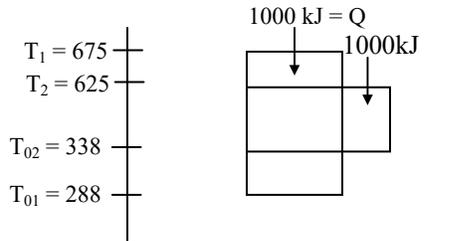
$$AE = Q \left( 1 - \frac{T_0}{T} \right) = 100 \left( 1 - \frac{288}{675} \right) = 57.33 \text{ kJ}$$
