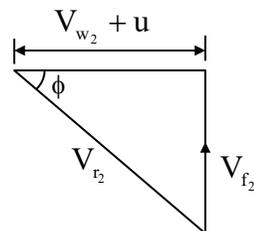
$$V_{w2} = V_{r2} \cos \phi - u$$
