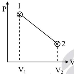
$${}_1W_2 = \frac{1}{2}(P_1 + P_2)V_s, \quad V_s = V_2 - V_1$$
