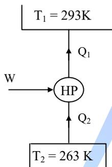
$$Q_1 = 0.65(T_1 - T_2) = 0.65(293 - 263) = 19.5 \text{ kW}$$
