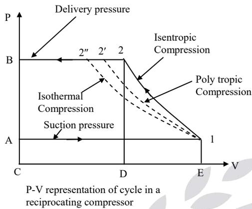
From the P.V. diagram we can see that work done is minimum when the compression process is isothermal.
