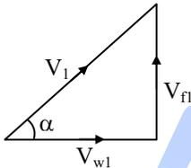
$$V_{w1} = V_1 \cos \alpha = 400 \cos 20^\circ = 375.87 \text{ m/s}$$
