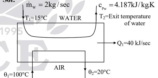
$$\dot{m}_a = 3 \text{ kg/sec}, \quad c_{p_a} = 1.005 \text{ kJ/kg.K}$$
