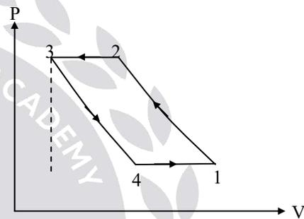
$$\text{Swept volume, } V_S = V_1 - V_3 = \frac{\pi}{4} \times D^2 \times L$$
