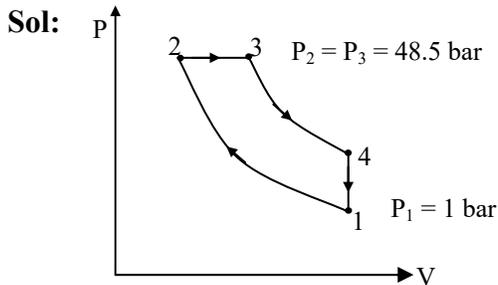
$$\text{Compression ratio} = r_k = \frac{V_1}{V_2}$$
