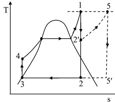
(i) Work output of turbine increases as expansion is carried in two stages.
