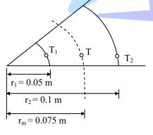
$$\frac{T_{m} - T_{1}}{T_{2} - T_{1}} = \frac{\frac{1}{r_{1}} - \frac{1}{r_{m}}}{\frac{1}{r_{1}} - \frac{1}{r_{2}}}$$
