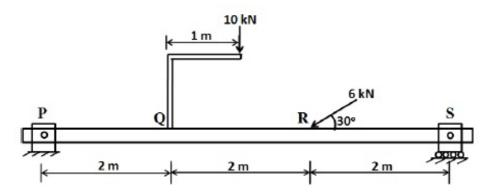
The bending moment, in Nm, at point R is \_\_\_\_\_.
