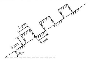
The theoretical R<sub>a</sub> value for this surface, in µm, is \_\_\_\_\_.
