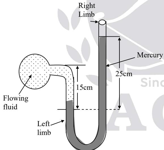
$P$  = pressure of the fluid in the pipe
