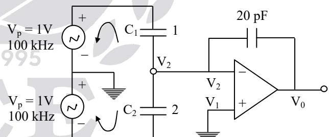
$V_1 = V_2$  Virtual ground concept
