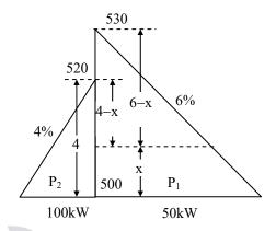
The no-load voltage of generator (A)
