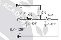
$$E\angle 0^{\circ} = \overline{V}_{Rs} - \frac{E}{2}\angle -120^{\circ}$$
