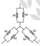
$$\begin{split} E_{ph} &= 4.44 \times 0.951 \times 0.957 \times 0.025 \times 50 \times 80 \\ &= 404 \ V \\ E_{L} &= \sqrt{3} \times E_{ph} = 700 \ V \end{split}$$
