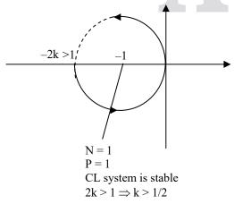
For k < 1/2, one closed loop pole in the right half of s-plane.
