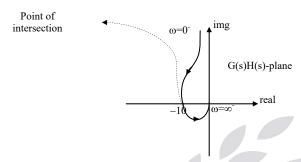
The mapping of the section  $C_1$  is shown figure.
