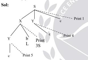
The depth first traversal of a parse tree generates an output 5, 3, 4, 1.
