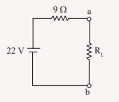
$$P_{\text{max}} = \frac{v_{\text{s}}^2}{4 \times 9} = \frac{(22)^2}{36} = 13.44 \text{ W}$$
