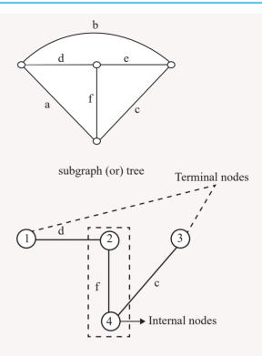
(2) & (4) are internal nodes which are incident exactly two branches
