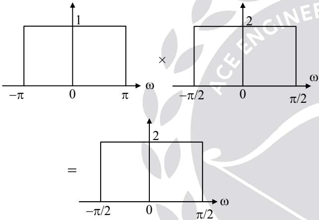
$$Y_3(\omega) = 2 \text{rect}\left(\frac{\omega}{\pi}\right)$$
