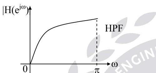
and it is FIR Filter because  $h(n)$  is finite duration.
