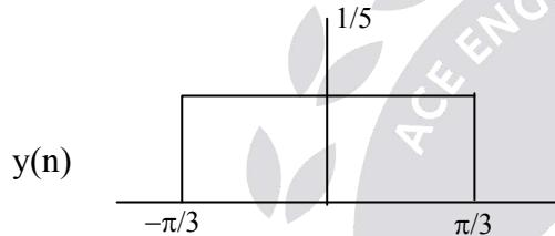
$$\sum_{n=-\infty}^{\infty} \frac{\sin \frac{n\pi}{4}}{2\pi n} \times \frac{\sin \frac{n\pi}{3}}{5\pi n} = \frac{1}{2\pi} \int_{-\frac{\pi}{4}}^{\frac{\pi}{4}} \left( \frac{1}{2} \right) \left( \frac{1}{5} \right) d\omega$$
