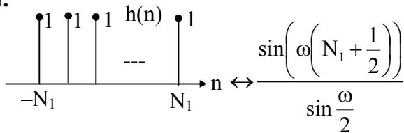
$$(a) H(\omega) = \frac{\sin\left(\frac{7\omega}{2}\right)}{\sin\left(\frac{\omega}{2}\right)}$$
