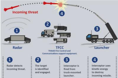
THAAD is coupled with space-based and ground-based surveillance stations, which transfer data about the
