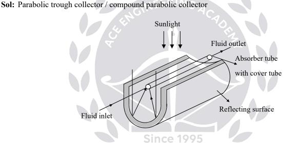
By proper tracking sun's rays are focussed on the absorber tube by which a fluid can be heated.
