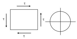
The corresponding Mohr circle should be concentric with origin.
