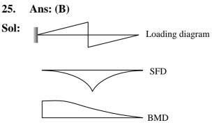
Slope of SFD = rate of loading and
