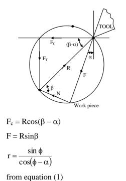
Fraction of energy with chip =  $\frac{F}{F_c} \times r$ =  $\frac{R \sin \beta}{R \cos(\beta - \alpha)} \times \frac{\sin \phi}{\cos(\phi - \alpha)}$ =  $\frac{\sin \phi \sin \beta}{\cos(\phi - \alpha)\cos(\beta - \alpha)}$
