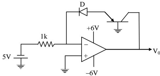
In this circuit diode tries to conduct but the transistor which is in cut-off region does not allow
