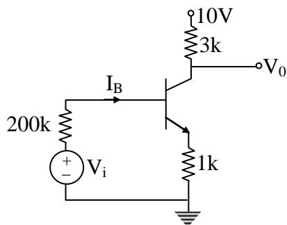
$$I_B = \frac{V_i - V_{BE}}{[200 + 1(1+\beta)] \times 10^3}$$
