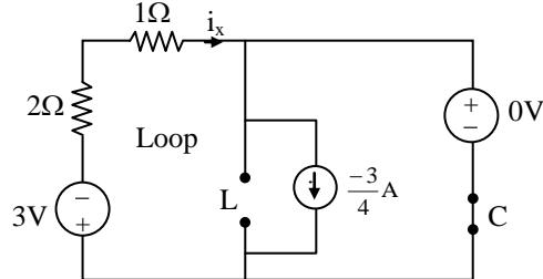
Applying kVL for the outer loop
