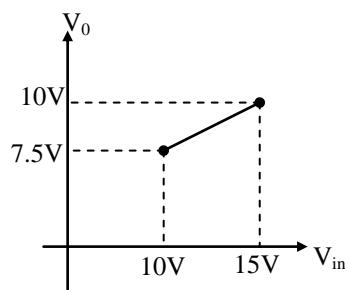
The slope of transfer characteristics
