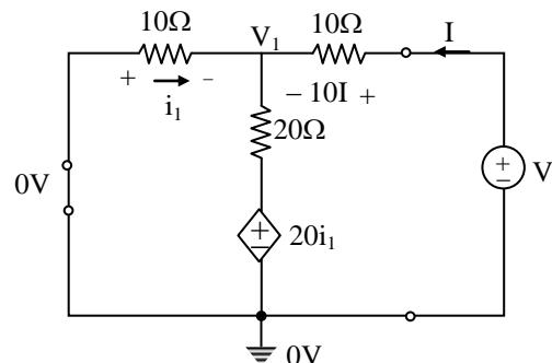
$$\text{By KVL} \Rightarrow 0 - 10i_1 - V_1 = 0 \Rightarrow V_1 = -10i_1 \quad \dots\dots (1)$$
