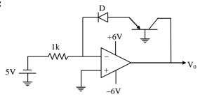
In this circuit diode tries to conduct but the transistor which is in cut-off region does not allow
