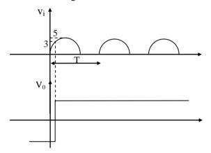
and Now if  $V_0$  becomes +10V, it will never come back to -10V since for that to happen V<sub>i</sub> should be less than -3 but given V<sub>i</sub> is always positive, so number of transitions is 1.
