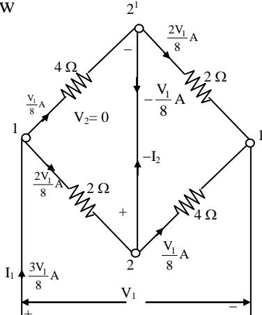
Between 1 and 1'; we have  $(4 \Omega // 2 \Omega)$  in series with  $(4 \Omega // 2 \Omega) = \frac{8}{3} \Omega$
