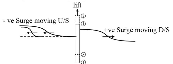
By lifting of gate, more discharge travel towards d/s. Hence +ve surge moving d/s and water levels falls on u/s, so -ve surge moving u/s.
