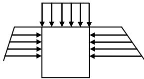
The force exerted by water will be due to the pressure on upper face as shown in the figure.
