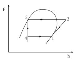
$$COP = \frac{RC}{P_{in}} = \frac{h_1 - h_4}{(h_2 - h_1)}$$
