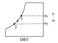
From the figure, it is clear that when warm saturated air is cooled
