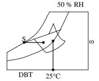
Lower DBT and higher relative humidity has less load.
