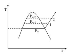
Partial pressure of vapour is very low and at low pressure water vapour can be treated as ideal gas irrespective of temperature.
