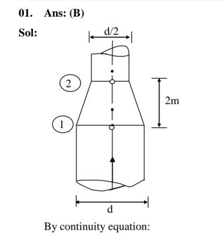
$$Q = A_1 V_1 = A_2 V_2$$
