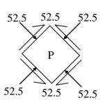
At plane ST,  $\sigma_x = \frac{-105}{2} = -52.5$  MPa  $\sigma_y = -52.5$  MPa  $\tau_{xy} = -52.5$  MPa
