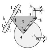
The links and the joints of the mechanism are labelled as illustrated in figure. The number of links is 5, the number of lower pairs  $(j_1)$  is 5, and the number of higher pairs  $(j_2)$  is 1.
