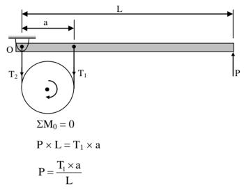
In simple band brake only two moments are acting about fulcrum  $\Rightarrow$  self energizing is not possible.
