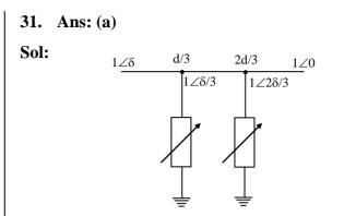
The steady state power transfer limit is  $P_m = \frac{1 \times 1}{0.1} = 10 \text{ pu}$
