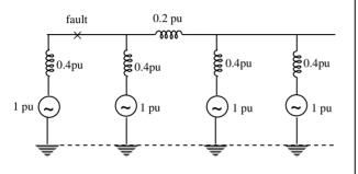
Equivalent reactance with respect to fault
