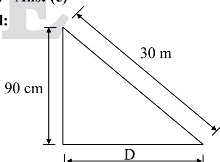
$$\begin{aligned} D &= \sqrt{(30)^2 - 0.9^2} \\ &= 29.986 \text{ cm} \end{aligned}$$
