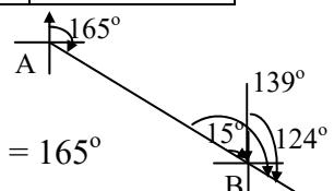
$$\text{Bearing of a line AB} = 165^\circ$$
