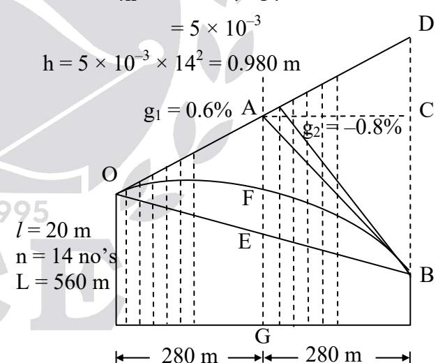
$$\text{RL of E} = \frac{1}{2} [\text{RL of O} + \text{RL of B}]$$
