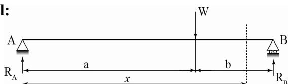
Consider a load 'W' on a simply supported beam AB of length ' $\ell$ ' at a distance 'a' from A.
