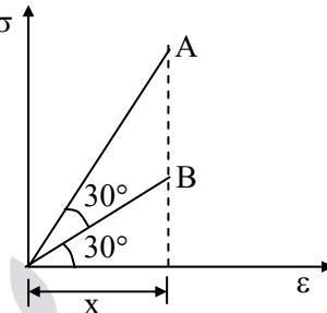
$$\frac{(SE)_A}{(SE)_B} = \frac{\text{Area under curve A}}{\text{Area under curve B}}$$
