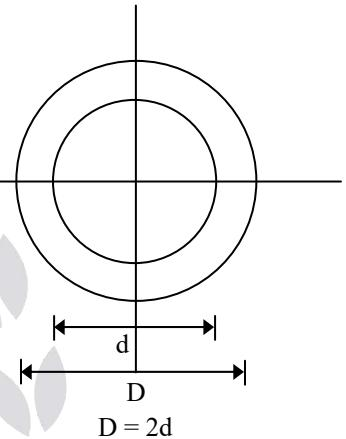
$$(Z_p)_{\text{solid}} = (Z_p)_{\text{hollow}}$$
