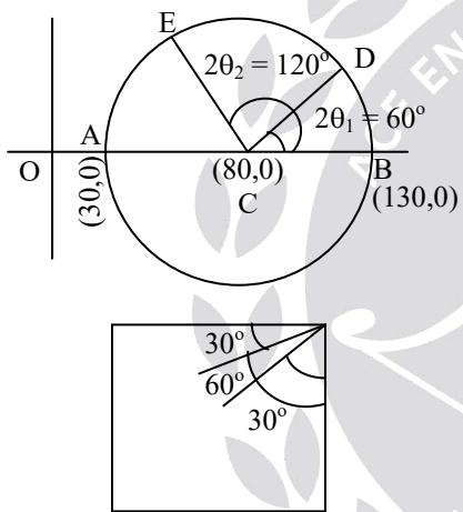
Stress on point inclined at  $30^\circ$  to y-axis in AC direction (Point D)
