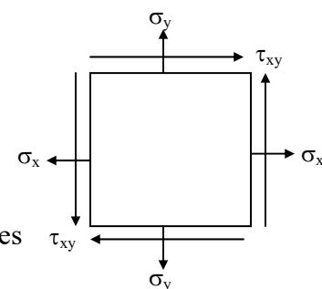
$$\sigma_1 \text{ and } \sigma_2 = \frac{\sigma_x + \sigma_y}{2} \pm \sqrt{\left(\frac{\sigma_x - \sigma_y}{2}\right)^2 + \tau_{xy}^2}$$
