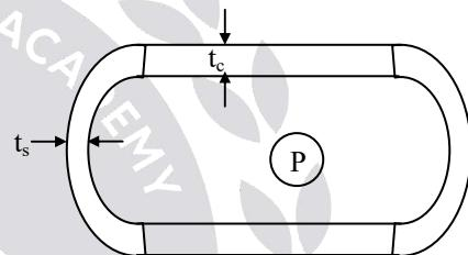
at the junction equal deformation is required
