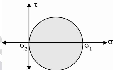
For any point above NA, and below extreme fiber Mohr's circle will be an intermediate of the above two cases i.e.,
