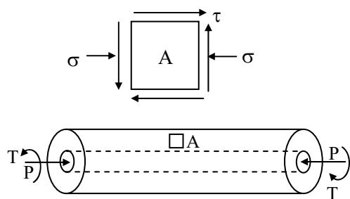
State of stress at any point on surface of shaft.
