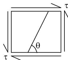
$\sigma_1 = \sigma_{\max}$ , at  $\theta = 45^\circ$  (maximum normal stress which causes failure of brittle material).
