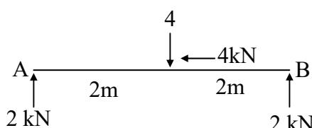
Reaction at both the supports are 2 kN and in upward direction.
