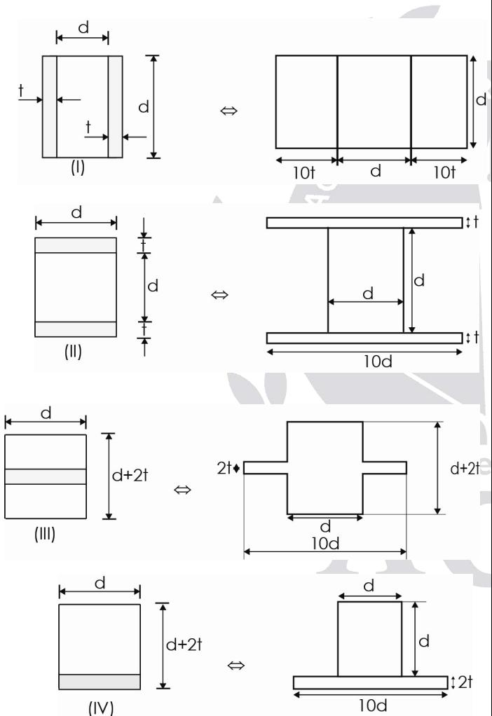
A beam that has larger section modulus will be stronger and support greater load.
