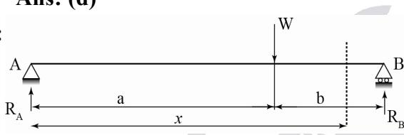
Consider a load 'W' on a simply supported beam AB of length ' $\ell$ ' at a distance 'a' from A.
