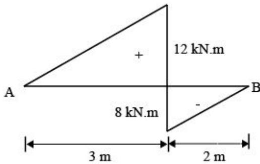
At section C there is a sudden change of BM, so there is a concentrated moment in AC direction at point C of magnitude  $12 - (-8) = 20 \text{ kNm}$
