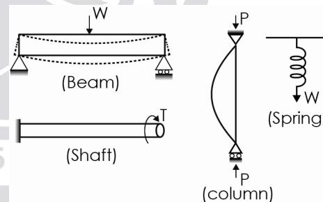
**Note:** When torque is applied to non circular sections, shear stress distribution is non-uniform and also warping occurs i.e. plane sections do not remain plane after twisting.
