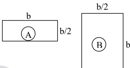
$$\text{By using flexural formula, } \sigma = \frac{M}{Z}$$
