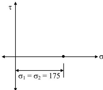
From the above, we can say that Mohr's circle is a point located at 175 MPa on normal stress axis.
