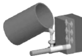
Shot sleeve filled With molten metal
