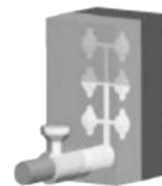
Piston forces molten Metal into the die
