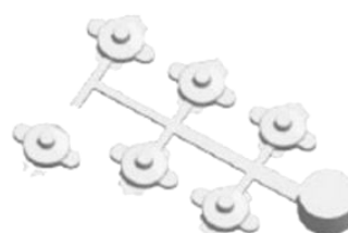
Individual cast parts are trimmed from the casting tree
