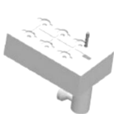
Die inserts machined From tool steel
