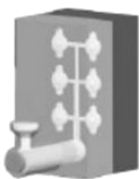
Piston maintains pressure on molten metal when die is filled
