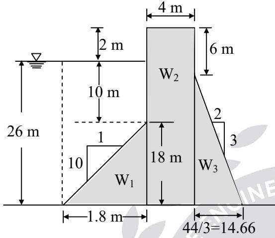
Ice force, wind force, seismic force need not be considered.
