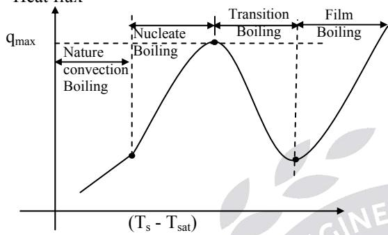
Temperature in nucleate boiling region is less than that of film boiling region as shown in figure.
