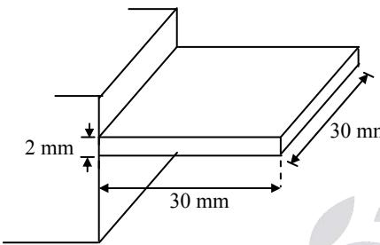
As the tip is not insulated at end, it loses heat from end also, hence the temperature variation for, heat dissipation from a fin loosing heat at tip also is given by
