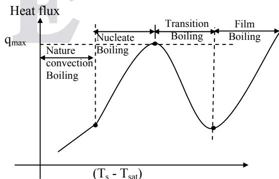
From above figure, with increase in temperature, the heat flux first increases upto critical point and then decreases and again it increases.
