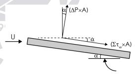
$F_D = (\Delta P \times A)\sin\alpha + (\Sigma \tau_w \times A)\cos\alpha$ Substituting the values given:
