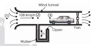
$$\frac{P_{1}}{\gamma_{air}} + \frac{V_{1}^{2}}{2g} + Z_{1} = \frac{P_{2}}{\gamma_{air}} + \frac{V_{2}^{2}}{2g} + Z_{2}$$
