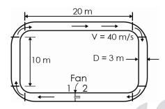
Applying Energy equation for two points, just upstream and downstream of the fan in the pipe loop.
