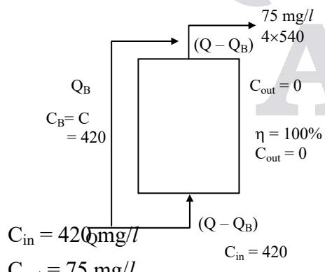
$$\eta = \frac{C_{in} - C_{out}}{C_{in}} \times 100 = \frac{420 - 75}{420} \times 100$$
