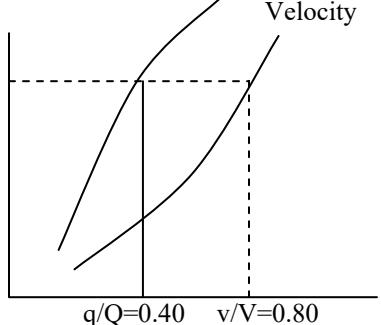
$$\text{Depth of flow} = 0.50D = 0.5 \times 0.30 \\ = 0.15 \text{ m} = 150 \text{ mm}$$
