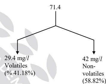
$$\frac{100}{S_{\text{solid}}} = \frac{\% \text{vol}}{S_{\text{volatile}}} + \frac{\% \text{non volatile}}{S_{\text{non volatile}}}$$
