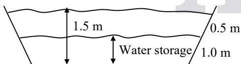
$$\text{Surface area of oxidation pond} = \frac{Q y_i}{\text{OLR}}$$
