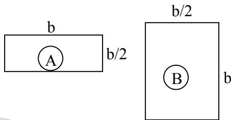
By using flexural formula,  $\sigma = \frac{M}{Z}$
