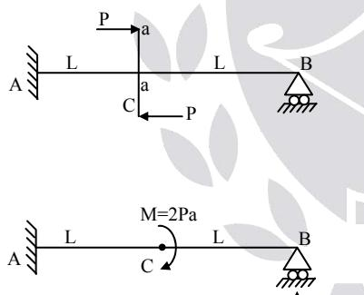
Applying, superposition principle
