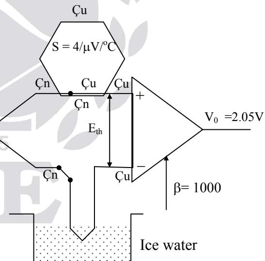
$$\therefore V_0 = \beta V_{in}$$
