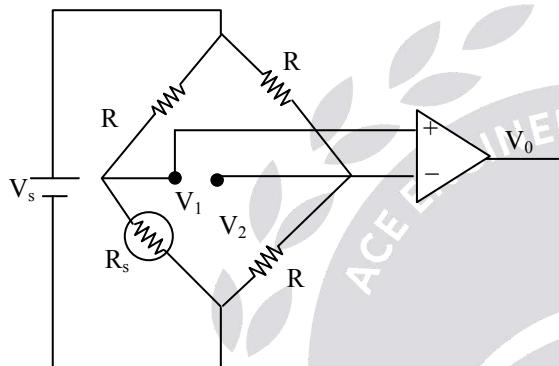
$$V_1 - V_2 = \frac{V_s \Delta R}{4R} \Rightarrow \frac{V_s}{4} \pm \frac{R \times \frac{1}{100}}{R}$$
