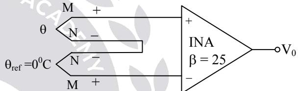
$$S = 40 \mu\text{V}/{}^{\circ}\text{C}$$
