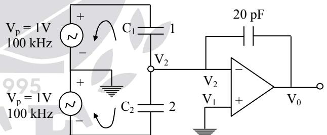
$V_1 = V_2$  Virtual ground concept
