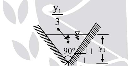
As it is not a rectangular channel, let us work out from fundamentals by equating specific force at the two sections.
