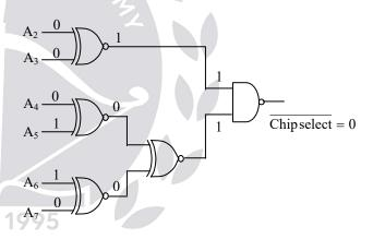
$\therefore$  Address space is 60H to 63H A<sub>o</sub> to A<sub>11</sub> are used for line selection A<sub>12</sub> to A<sub>15</sub> are used for chip selection
