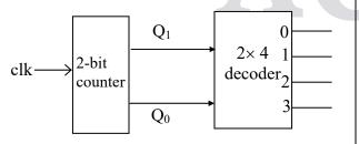
Outputs of counter is connected to inputs of decoder
