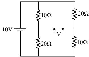
$$V = V_+ - V_-$$
