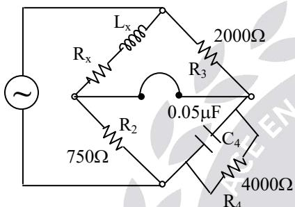
$$\frac{L_x}{C_4} = R_2 R_3$$
