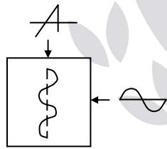
∴ Two cycles of sine wave displayed on vertical time base
