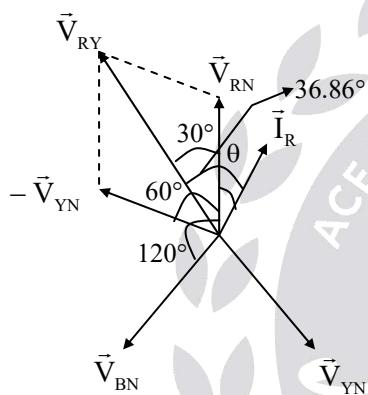
Current coil is connected in 'R<sub>phase</sub>', it reads ' $\vec{I}_R$ ', current.
