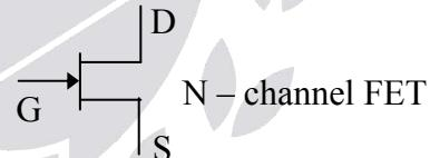
Input resistance of FET is of the order of tens (or) hundreds of mega ohms ( $M\Omega$ s)
