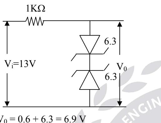
$$V_0 = 0.6 + 6.3 = 6.9 \text{ V}$$
