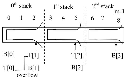
$$\left. \begin{aligned} T[0] &= B[1] \\ T[1] &= B[2] \\ T[2] &= B[3] \end{aligned} \right\} \text{ overflow cases}$$
