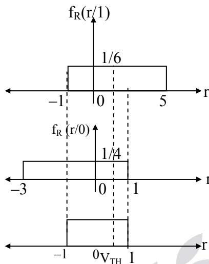
For minimum error the  $V_{TH}$  should lie in the area of intersection of the 2 pdf's.
