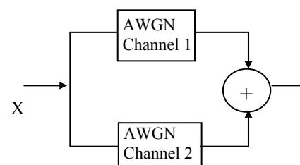
At the input of the receiver signal amplitude is doubled. But when two independent Gaussian Random Variables are added, the resultant random variables is also a Gaussian random. The pdf is the convolution of individual pdf's.
