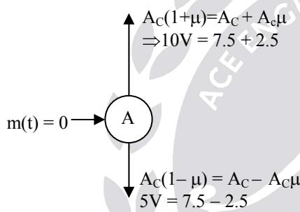
$$\text{Amplitude deviation } A_C\mu = 7.5 \times \frac{1}{3} = 2.5 V$$
