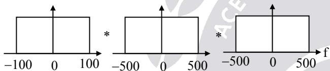
So, highest frequency component in the signal  $m(t)$  is  $100 + 500 + 500 = 1100$
