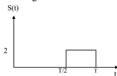
$$\begin{aligned}\Rightarrow S_0(t)_{\max} &= \int_{T/2}^T 2^2 dt \\ &= 4 \int_{T/2}^T 1 dt \\ &= 4[T - T/2] \\ &= 2T\end{aligned}$$
