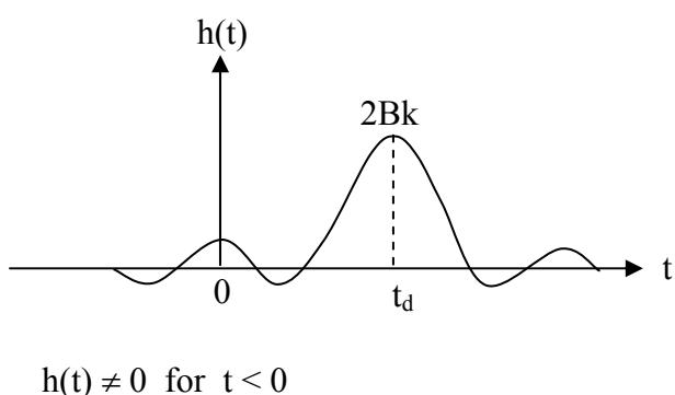
Output exists before input is applied i.e. non-causal, which is physically impossible.
