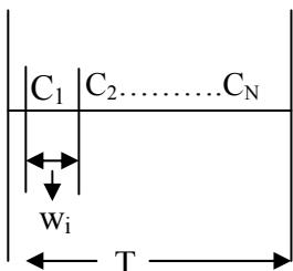
$$\text{Minimum B.W of TDM is } \sum_{i=1}^N w_i$$
