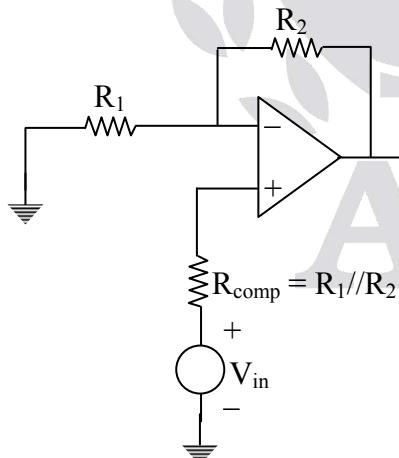
$$\begin{aligned} \rightarrow R_{\text{comp}} &= R_1//R_2, \text{ then } V_0 = (I_{B1} - I_{B2}) R_2 \\ &= I_{os} R_2 \\ V_0 &= (I_{B1} - I_{B2}) R_2 \\ &= I_{os} R_2 \\ &= 1/10 (I_B R_2) \end{aligned}$$
