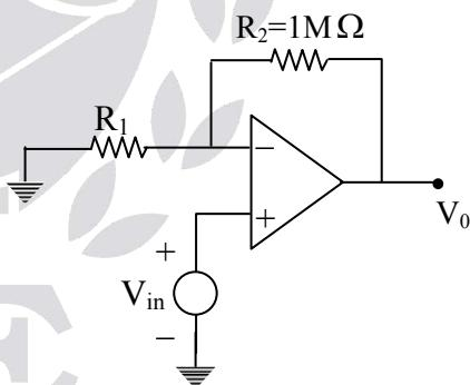
$$\text{Gain} = \frac{V_0}{V_{in}} = 1 + \frac{1\text{M}}{R_1} = 100 \Rightarrow R_1 = 10.1 \text{ k}\Omega$$
