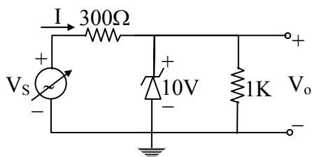
$$I_z = 1\text{mA} \text{ to } 60\text{mA}$$
