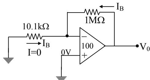
$$\begin{aligned} V_0 &= I_B(1M) \\ &= 100nA(1M) \\ &= 0.1V \end{aligned}$$
