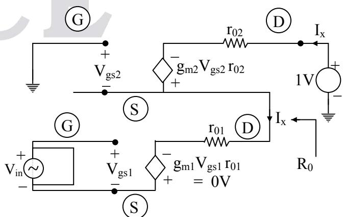
By KVL  $V_{gs2} + I_x r_{01} = 0$
