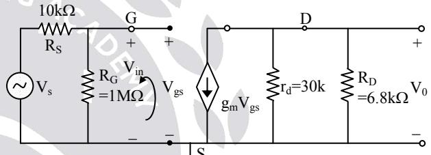
$$V_0 = -g_m V_{gs} (r_d \| R_D)$$
