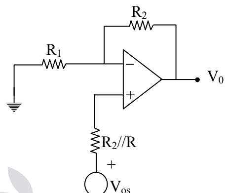
$$\begin{aligned} V_0 &= |V_{0_{\text{Offset Voltage}}}| + |V_{0_{\text{Bias current}}}| \\ &= 0.1 + 0.01 \\ &= 0.11 \end{aligned}$$
