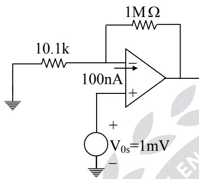
$$\begin{aligned} V_0 &= |V_{0_{\text{Bias current}}}| + |V_{0_{\text{Offset Voltage}}}| \\ &= 1M(I_B) + \left(1 + \frac{R_2}{R_1}\right)V_{os} \\ &= 1M(100nA) + 100(1mV) \\ &= 0.2V \end{aligned}$$
