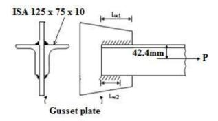
The C.G of an angle located at a distance 42.4 mm from edge of an angle
