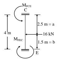
The fixed end moments (FEMS) have been worked out on the approximation that the 4 'beams' in the frame act independently. Ends BA, BC, CB, CD, DC, & CE are not really fixed ends. They are assumed to be, as a first approximation in the moment distribution process.
