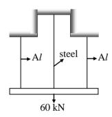
As the Bar is rigid, elongation in each wire will be same. Let load P is carried by aluminimum wire.
