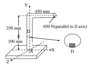
As point 'D' is on the extreme fiber of the cross section
