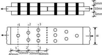
The width of main plate and cover plate can be computed based on tensile strength of main plate and cover plate at section 1-1 and section 3-3 respectively
