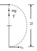
The forces acting on the bob at the highest point+ are mg due to the gravity and T due to the tension in the string. The resultant force towards the centre is, therefore, mg + T. As the bob is moving in a circle, its acceleration towards the centre is  $v^2/l$ . Applying Newton's second law and using (i),
