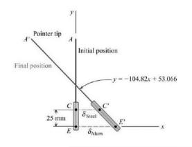
Take the initial position of E as the origin. The coordinates of E in the deflected position are (0.50625 mm, 0) and the coordinates of C are (0.267750 mm, 25 mm). Use the deflected position coordinates of E and C to determine the slope of the pointer.
