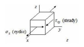
This is relatively simple state of stress and the principal stress can be determined from Mohr's circle. Since it is a state of plane stress, we know that  $\sigma_{eq} = \sqrt{\sigma_x^2 + 3\tau_{xy}^2}$ ,
