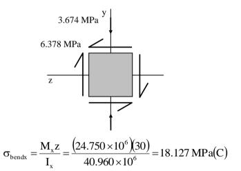
Bending stress at K due to M<sub>z</sub>:
